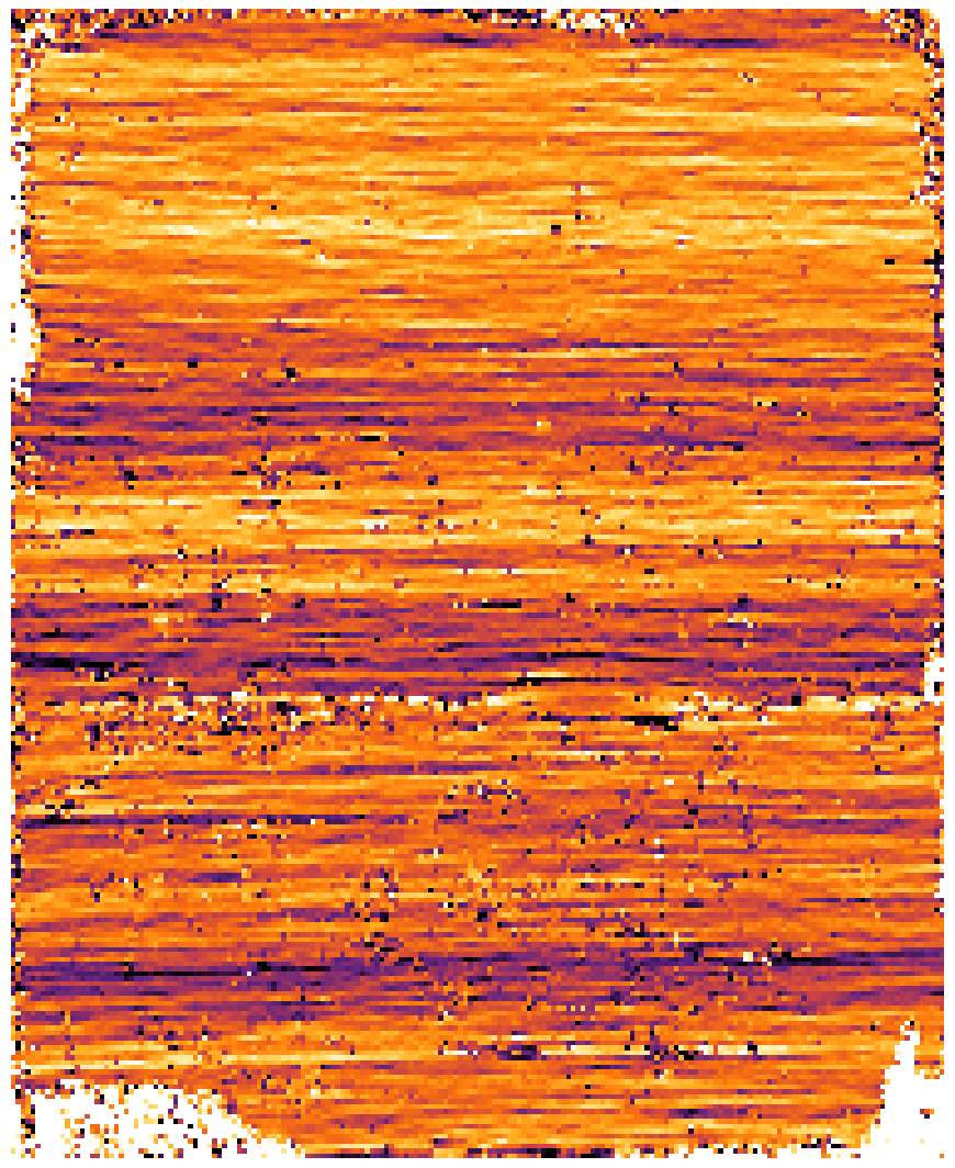
horizontal thread density (11.81 +/- 1.34 threads/cm)
